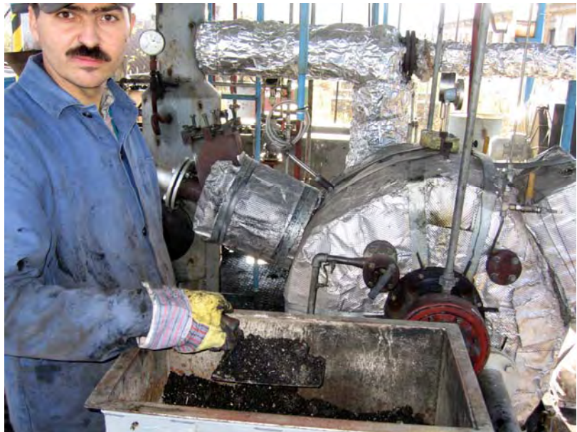
Bitumen sand processing test in the Blowdec 45 kW unit
